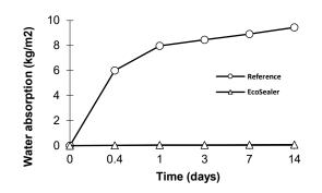
Water Absorption of Treated Brick
